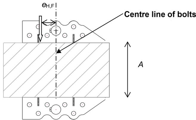
The minimum value of the following formulas and also formula [Eq.11] for the characteristic lateral load-carrying capacity of the joist hanger connection applies to a joist hanger with 2 bolts.
