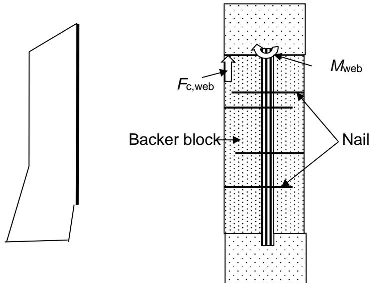
Static model for a vertical force downward. The header beam has been drawn a little away to the right to show the forces acting. The header is shown with the forces and moment acting on it.
