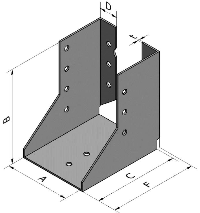
Parameters have to be used with equation in [Annex C](#) **$k_{H,1}$  for Joist Hanger SAI 1st blank model - Full nailing - F1**
