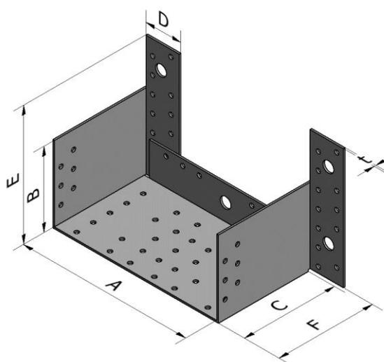
**Characteristic capacity for ETC G/D - Full nailing - F1 - timber to timber**
