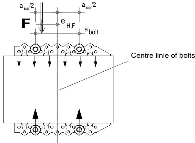
For a lateral force the formula for the characteristic load-carrying capacity of the joist hanger connection with 4 Ø10 mm bolts is:
