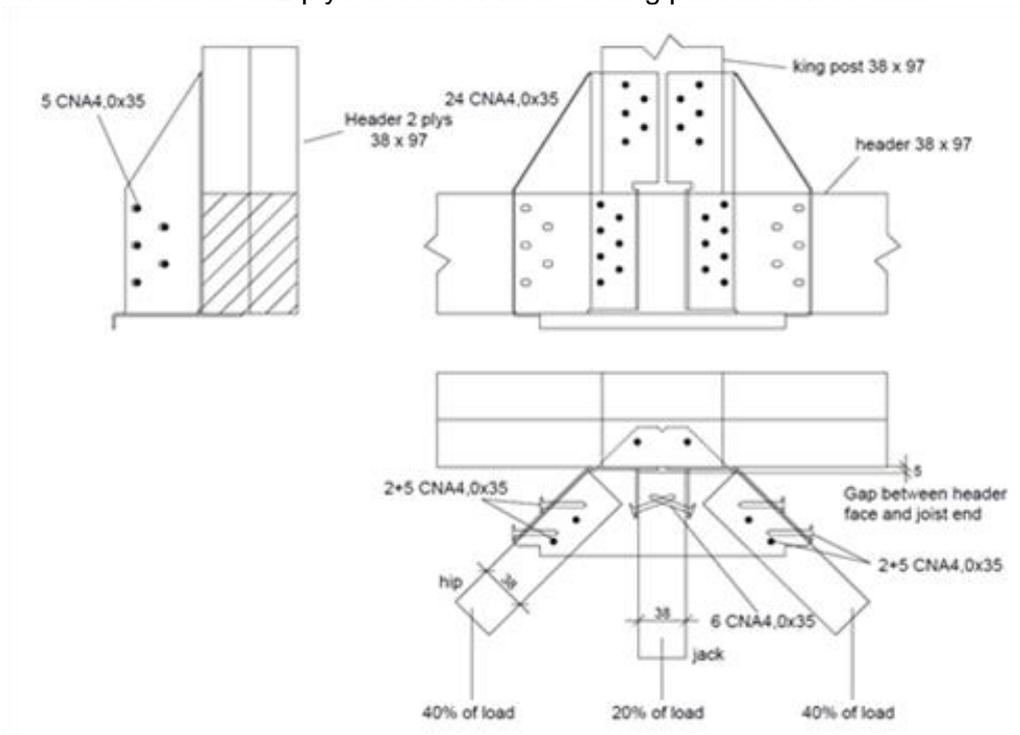
**Characteristic capacity for ETC - Full nailing - F1, F2 - timber to timber - 1 jack + 1 hip**
