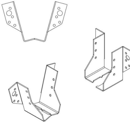
Picture below shows, on the left hand side, a joist hanger installed on a 45 mm width joist (1 element), and on the right hand side, a joist hanger installed on a 80 mm width joist, where the joist hanger has been splitted into 2 elements.
