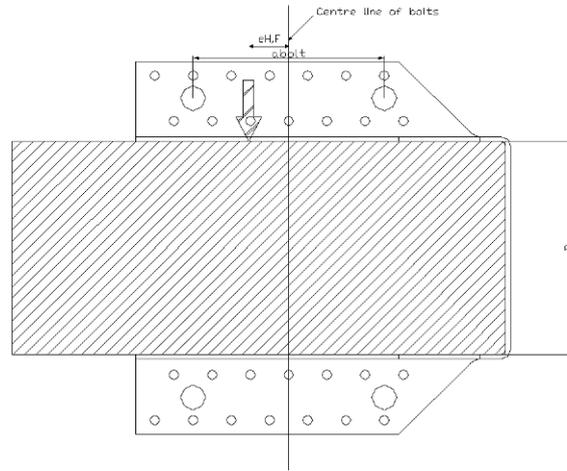
Provided the force is acting between the anchor bolts the characteristic lateral load-carrying capacity of the joist hanger connection with 4 Ø12 mm bolts is:
