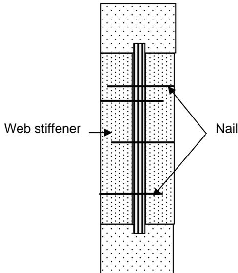
Web stiffeners on the joist at the joist hanger. The web stiffener shall fit to the bottom flange and have a width of 2/3 of the height between the inner sides of the flanges.
