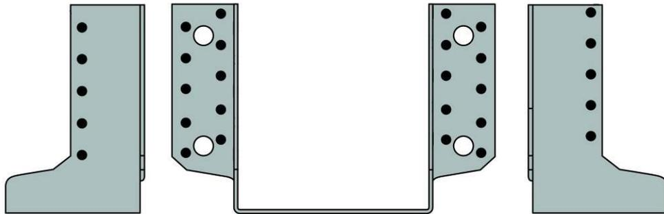
Fill it in all the holes with nails, on the face and the side flanges.
