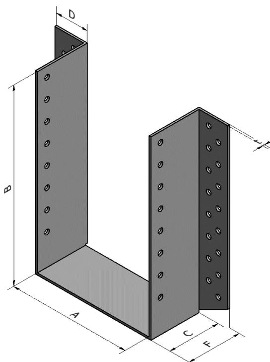
Special version - bolt holes, holes in the seat, asymmetric holes in the sides
