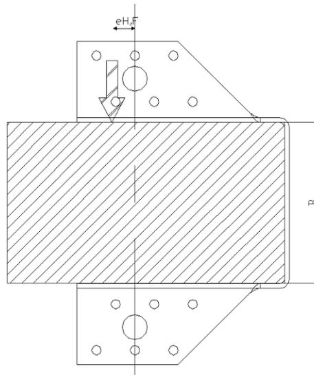
Provided the joist is prevented from rotation around its own axis, i.e. the force is acting right at the anchor bolts with  $e_{H,F} = 0$  mm the characteristic lateral load-carrying capacity of the joist hanger connection with 2 Ø12 mm bolts is:
