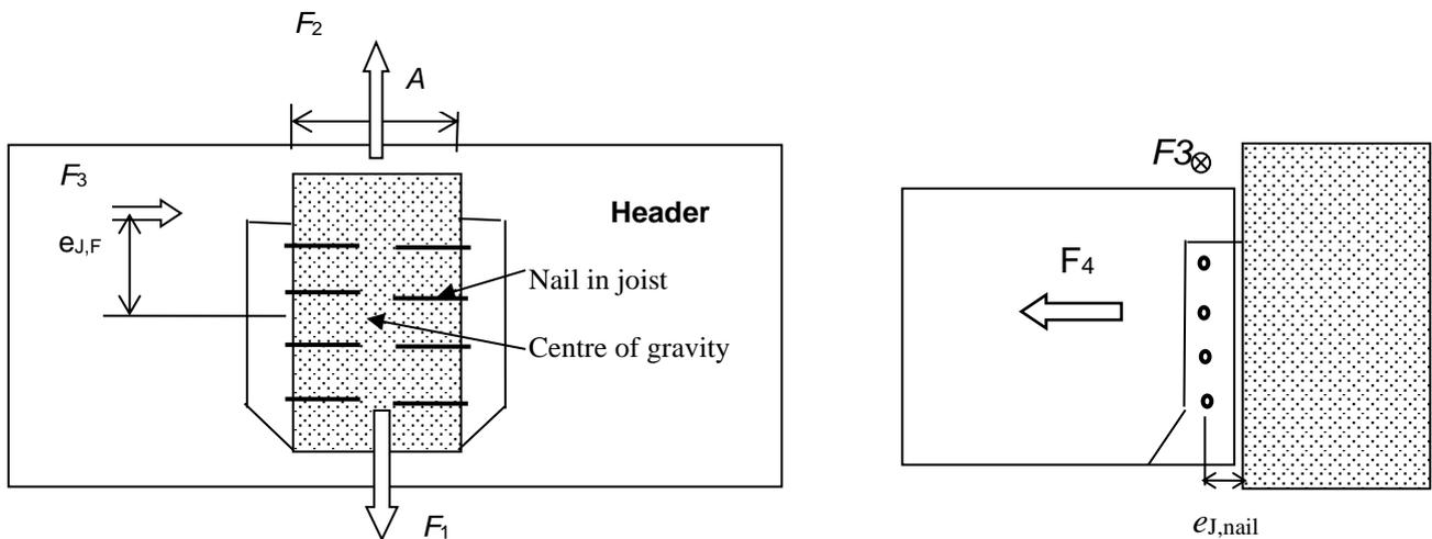
**Figure 1:** Definition of  $F_1$ ,  $F_2$ ,  $F_3$ ,  $F_4$ ,  $e_{j,F}$  and  $e_{j,nail}$
