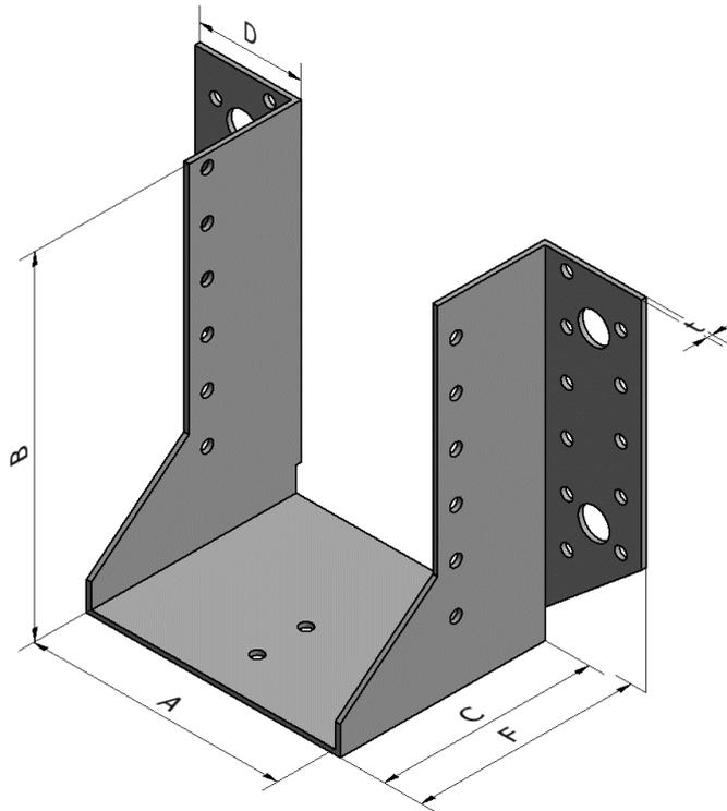
Parameters have to be used with equation in [Annex C](#). **$k_{H,1}$  for Joist Hanger SAE - Full nailing - F1**
