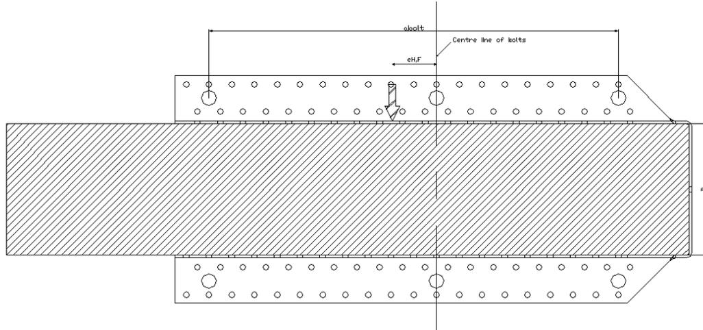
Provided the force is acting between the outer anchor bolts and the force is acting  $e_{H,F}$  from the middle anchor bolt the characteristic lateral load-carrying capacity of the joist hanger connection with 6 12 mm bolts is:
