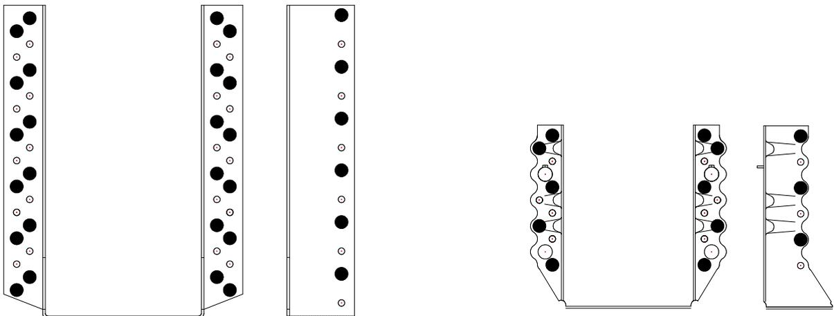
For all joist hangers, partial nailing capacities are also valid for joists connected on column as soon as the specific nailing pattern shown above is fulfilled.
