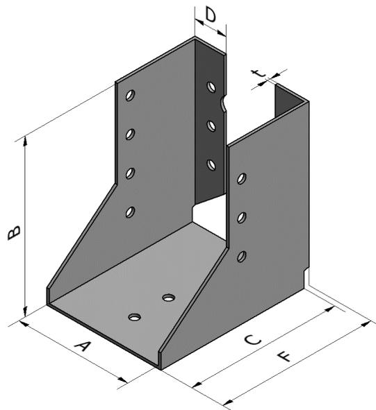
**k<sub>H,1</sub> for Joist Hanger SAIX - Partial nailing - F1**
