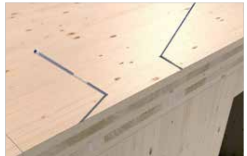
SWD inclined installation of CLT floor panels.
